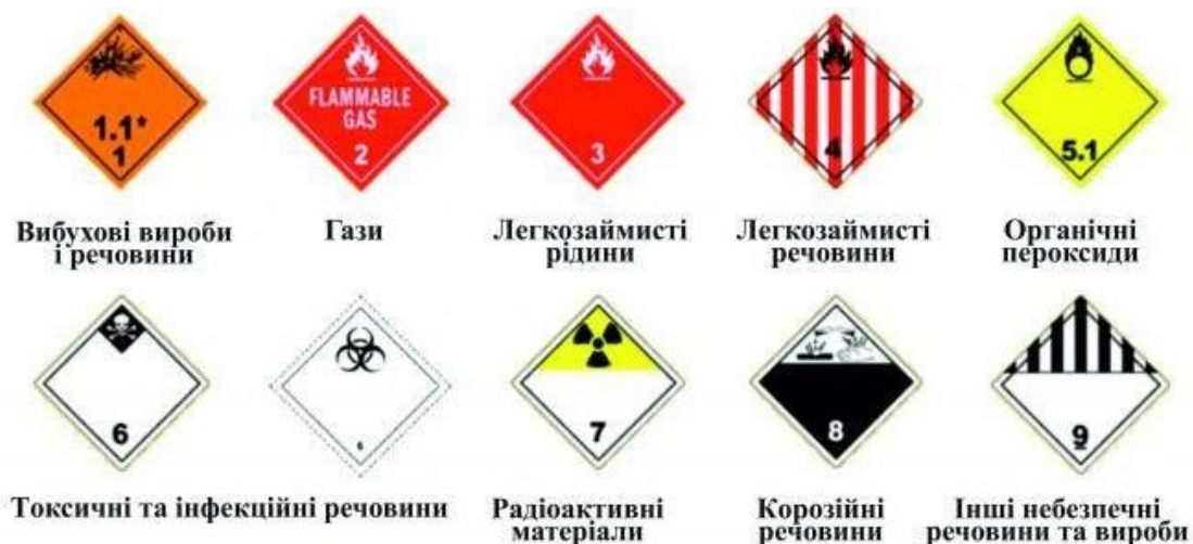
Figure 1 – Marking of dangerous goods
