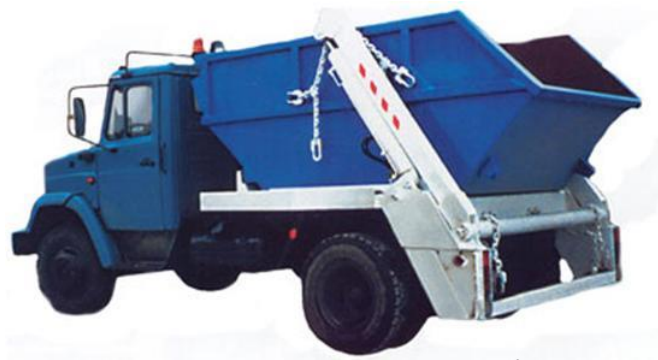
Fig. 3. Container garbage truck for containers with a volume of 7.6 m 3 for collecting large-sized waste
