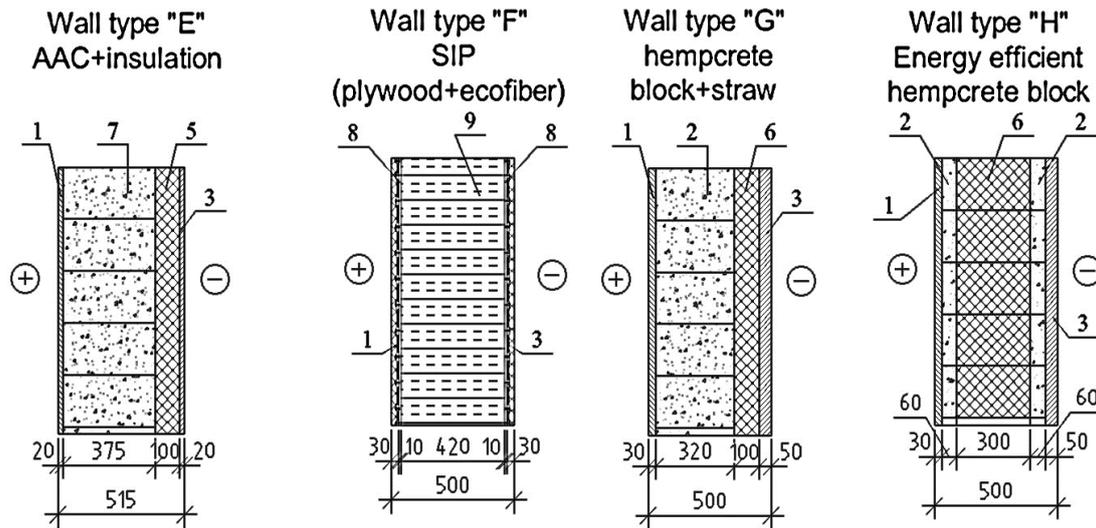
Fig 2. Considered wall types compositions «E»-«H» (1 – internal lime-sand plaster, 2 – hemcrete, 3 – external lime-sand plaster, 4 – honeycomb brick, 5 – mineral wool, 6 – strawbale panel, 7 – autoclaved aerated concrete (AAC), 8 – plywood, 9 – ecofiber)
